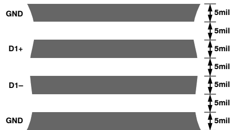
Figure 17. Arrangements of Signal Tracks
